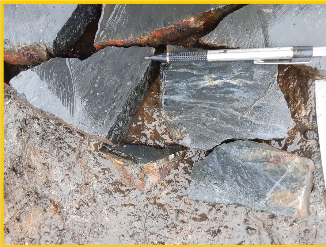
Figure 23a. Mineralized basalt/andesite with irregular felsic veins and trace garnet, trench 20-STR06a, GoldenEye prospect, north Sakami property, James Bay Territory.
