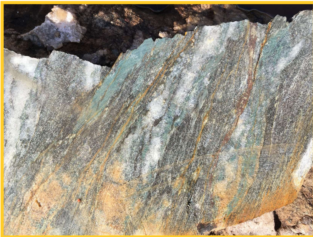
Figure 21a. Cm-thick pyrite-sphalerite vein with traces of chalcopyrite in a chlorite-metagreywacke, trench no. 20-STR03.
