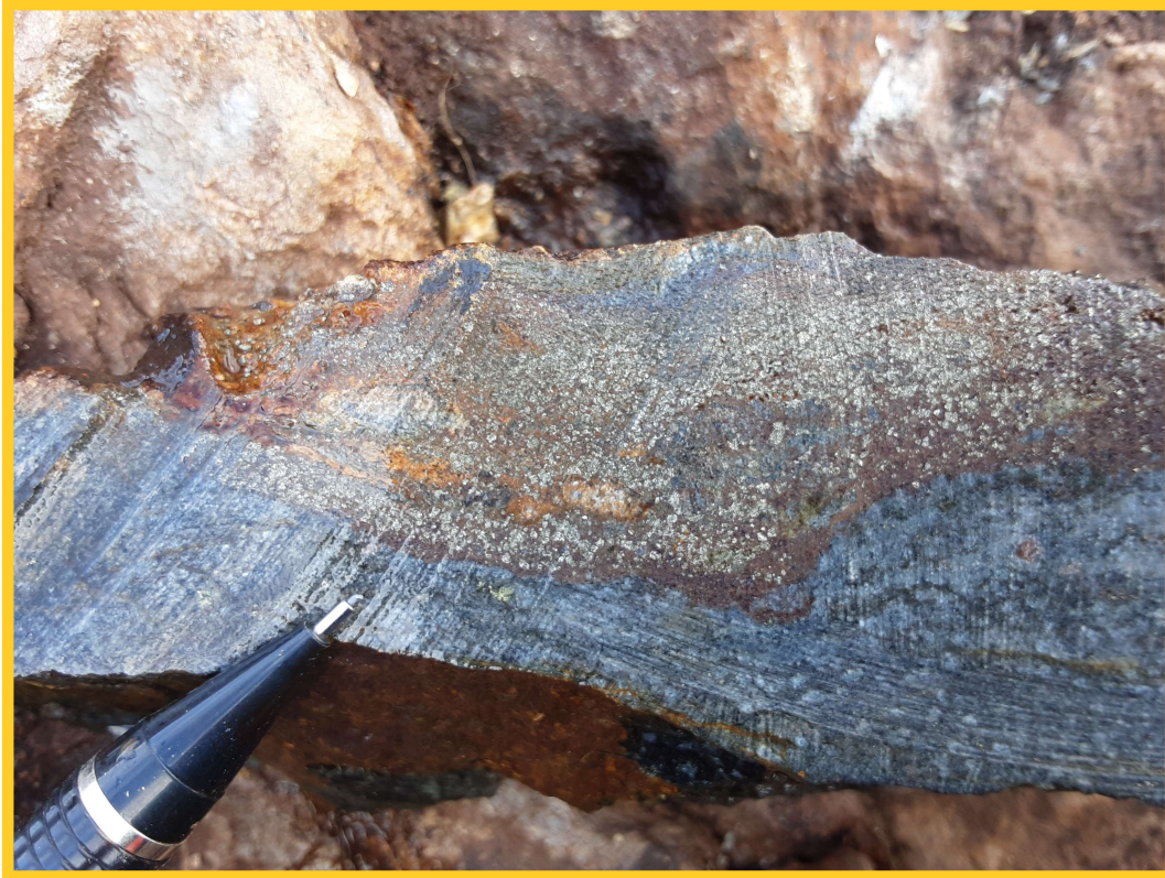
Figure 21a. Cm-thick pyrite-sphalerite vein with traces of chalcopyrite in a chlorite-metagreywacke, trench no. 20-STR03.
